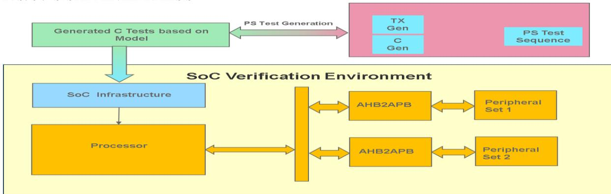
Figure12: PS Model reuse at SoC level Verification
