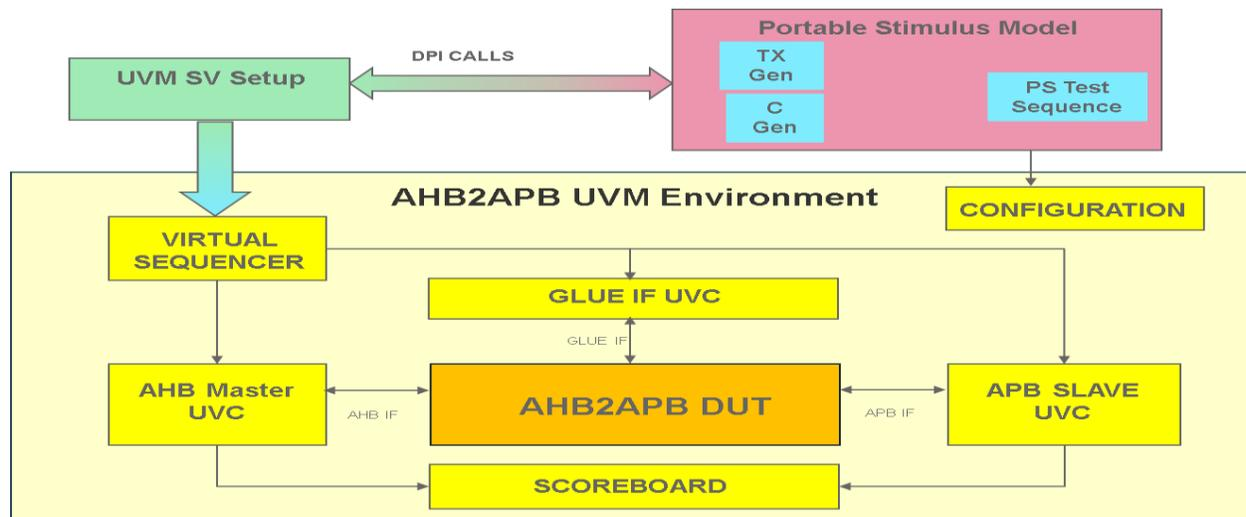
Figure9: AHB2APB Gasket PS based environment
