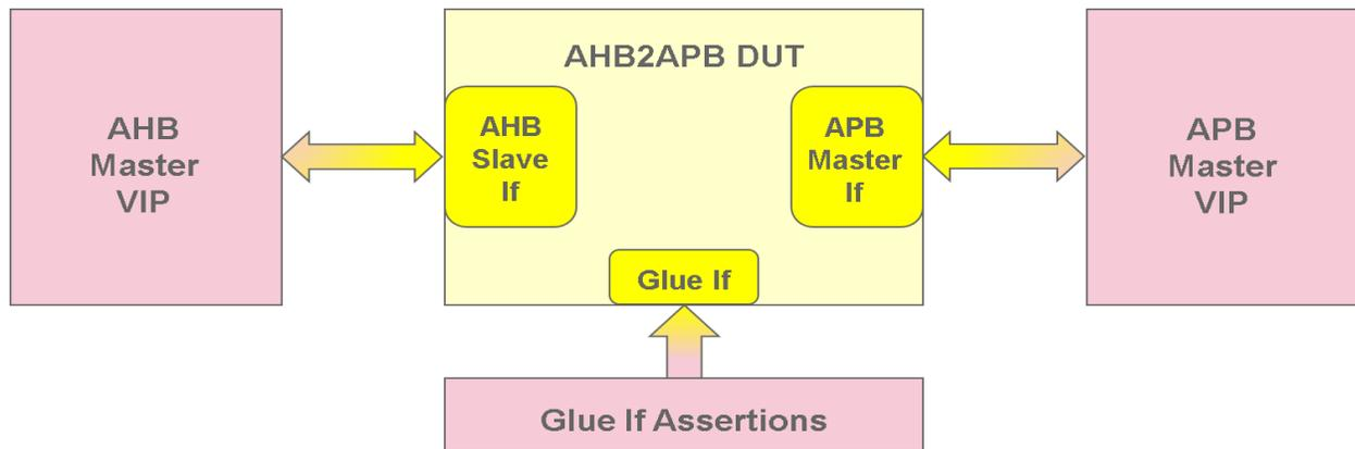
Figure6: AHB2APB Gasket Formal Verification environment
