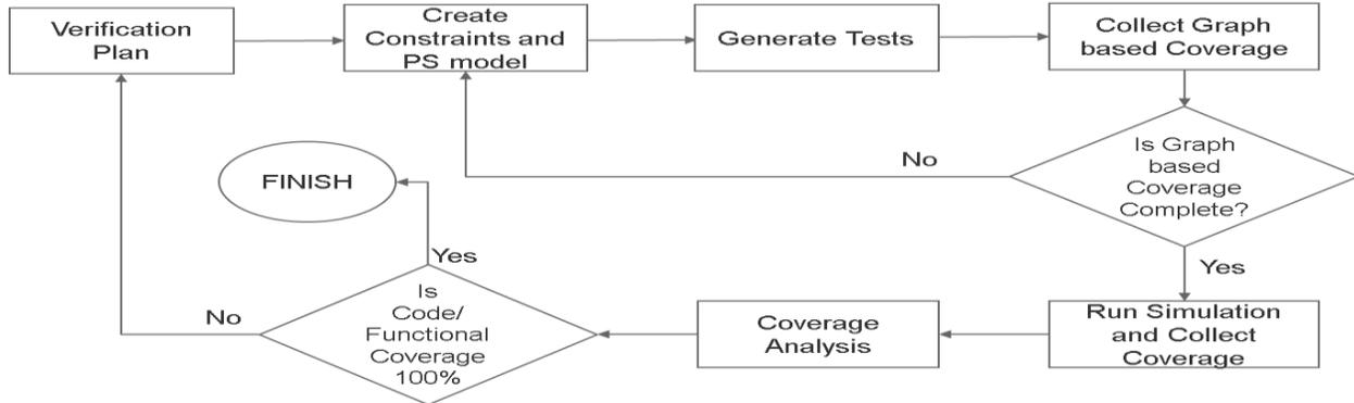
Figure8: Verification Flow with Portable Stimulus
