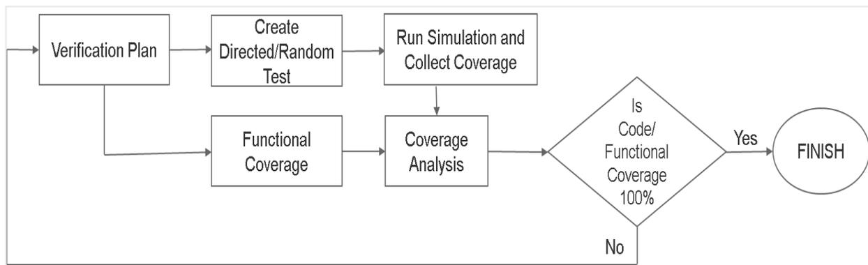
Figure2: Verification Flow with UVM
