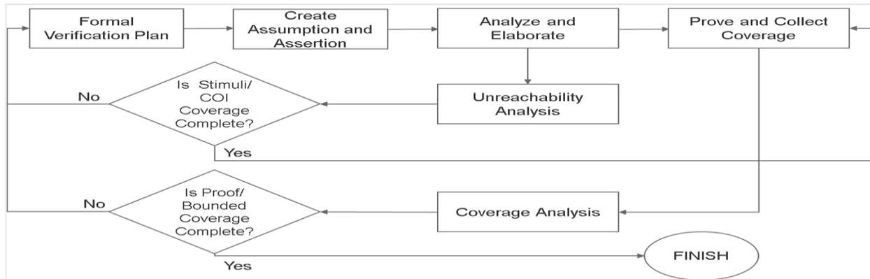
Figure4: Verification Flow with Formal
