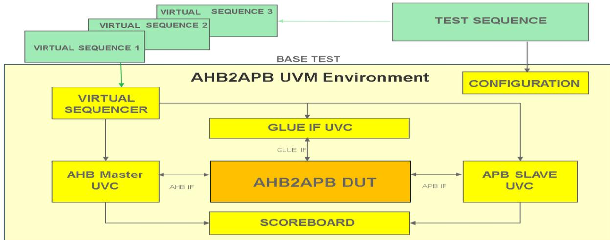
Figure3: AHB2APB Gasket UVM based environment
